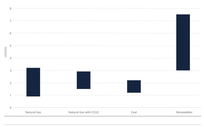
The cost of green hydrogen depends on the cost of the renewable power. An electrolyzer is a black box for converting renewable electrons into renewable molecules. The cost that dominates is the levelized cost of electricity (LCOE)<sup>2</sup>. The capex of electrolyzers and load factor are secondary to the LCOE." That optimistic view places primary emphasis on achieving increased volumes alongside decreased process and power costs; in the view of many there is a route to achieving those goals.
